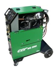
CARMIG 2000: place of deposit for welding torch PP100 for MIG aluminiumwelding
